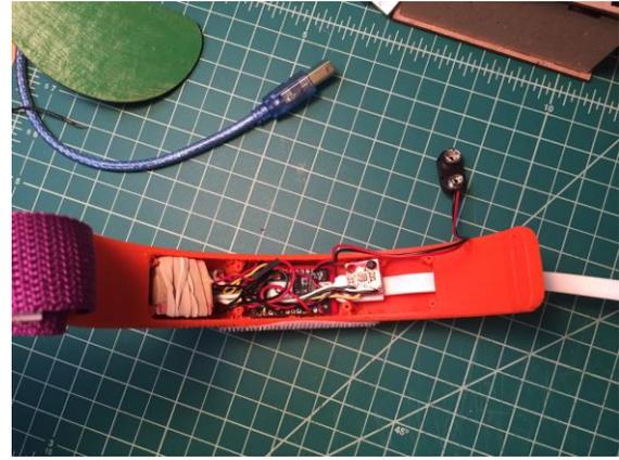
Fig. 2. Ambient sound and light sensors, as well as a motion sensor, were embedded in a collar worn by Paro during the intervention.
