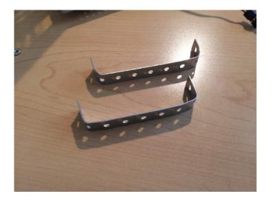
We then attach these to the back side of the face/head. Note, that the top Arduino support goes 4 holes down the arm from where the eye supports attached, and the bottom Arduino support goes 8 holes up the arm from where the mouth supports attached. This spacing is important for the holes on the Arduino to line up correctly so that you can attach it with screws.
