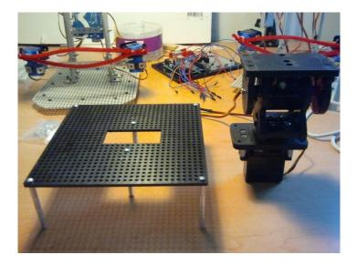
We then attach the Pan&Tilt system to the plate, using a couple screw/nuts.
