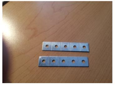
Then we need to bend them between the 4<sup>th</sup> and 5<sup>th</sup> hole. Make sure the 5<sup>th</sup> hole is flat, so it can be secured flush against the eye support.
